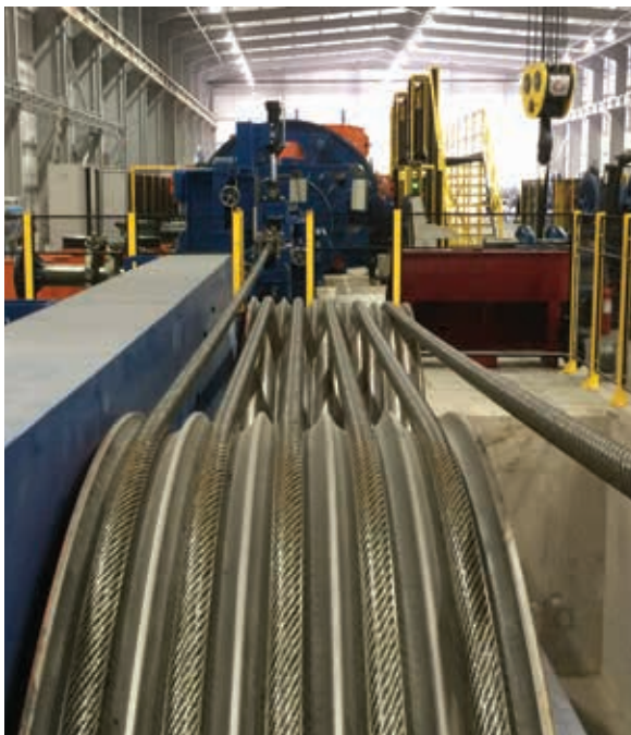
Wire rope production and rope sample after retirement (complete rope, rope core and retention system)
